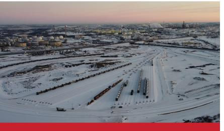
**CANDO SOUTHLANDS TERMINAL:** contracted in 2022 by Imperial to design-build-finance-operate-maintain a terminal in Strathcona, AB - completed in Q4 of 2024 on time and on budget - adds more than 600 additional operational and railcar storage spaces, utilizing both loop and ladder tracks to connect to both of Canada's Class I railways.
