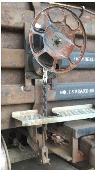
Bell crank in released position
