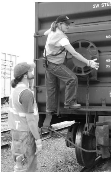
Operating Employee utilizing 3-point Contact for applying a vertical handbrake
