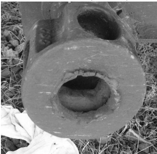
Damaged capstan (rounded square drive socket)
